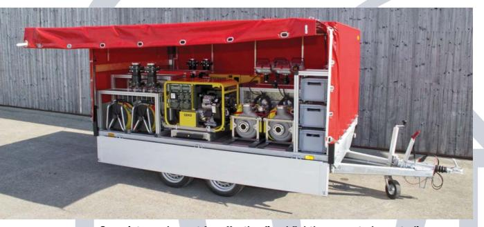
Complete equipment for effective flood fighting mounted on a trailer The equipment of the flood challenge trailer can be used independently on two different sites. Each of the 2 generators is able to operate 2 WOODY pumps. The total pump capacity of the trailer is 6400 l/min.
